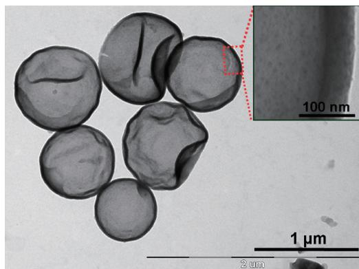
**Figure 1.** TEM images showing the morphology of hybrid hollow microspheres. The weight ratio of St/TEOS/MPS/HD/PSt is 10.0/12.0/1.2/0.8/0.2 (Sample 5 shown in Table S1<sup>10</sup>).
