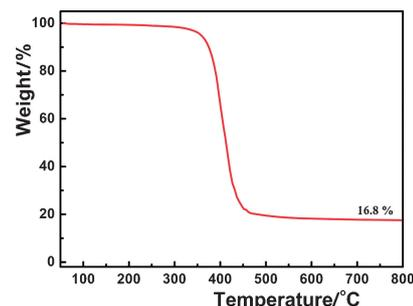
**Figure 3.** TGA curve of hybrid hollow microspheres.
