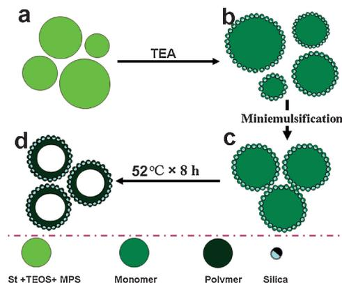
**Scheme 1.** Schematic illustration for the preparation of hybrid microcapsules via in situ Pickering miniemulsion polymerization.
